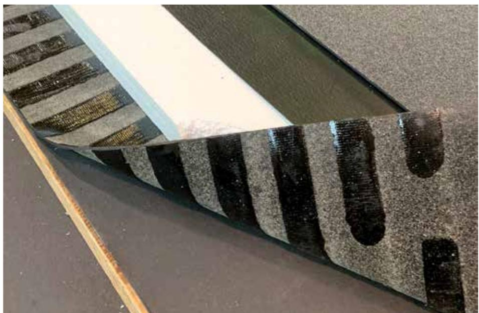
The same pattern of strips on the face of the membrane gives excellent bonding – strong and elastic.
